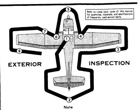
Visually check aircraft for general condition during walkaround inspection. In cold weather, remove even small accumulations of frost, ice or snow from wing, tail and control surfaces. Also, make sure that control surfaces contain no internal accumulations of ice or debris. If night flight is planned, check operation of all lights, and make sure a flashlight is available.
