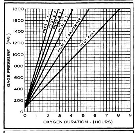
NOTE: This chart is based on a pilot with an orange color-coded oxygen line fitting and passengers with green color-coded line fittings.
